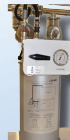
External solvent vapor removal
